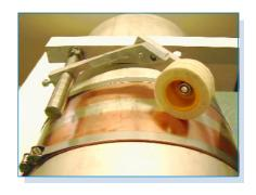
Constant contamination of silver surface increase the risk of spark erosion due to bad contact. Continous **Slipring Cleaning Device** prevents increase of the residual potential and keeps **JOWA - PES** in safe condition over long time.
