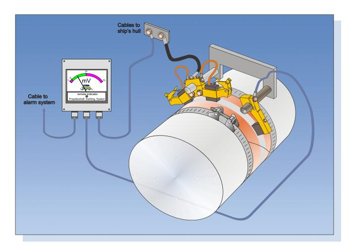
The high efficient **JOWA - PES** provides best protection against spark erosion, generated between dissimilar materials of rotating propeller (made of bronze) and steel hull being immersed in sea water.
