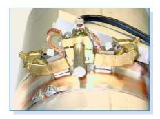
**JOWA - PES** protects the exposed propeller and bearings against galvanic or spark erosion damages. High efficiency silver tracked sliprings and proven contact brushes ensure a short circuit between the rotating propeller shaft and the ship's hull.
